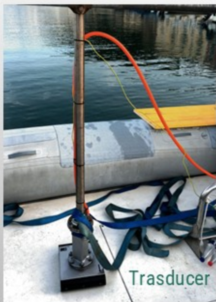
Attached onto an iron pole fastened to the side of a rubber boat
