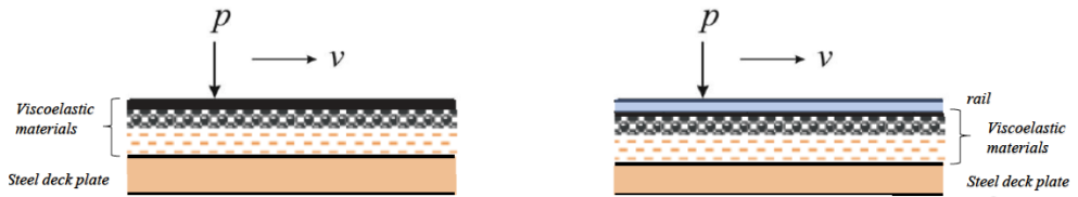
Fig. 2 - Schematic view of a load p moving with velocity v : roadway system, on the left, and rail system, on the right.
